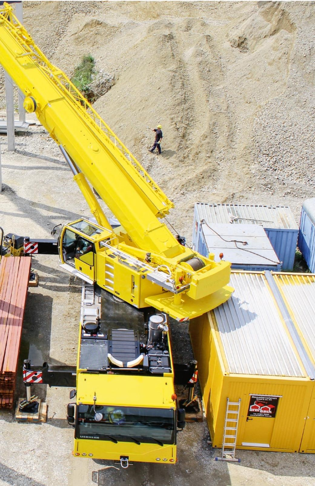
Working on sites often means constricted conditions. It is frequently impossible to extend all the supports on the mobile crane evenly. VarioBase® from Liebherr allows the crane to be used safely and flexibly in these difficult conditions. VarioBase® also provides higher load capacities and a larger working range in most working positions.
